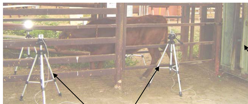
Two light beams measure animal's flight time
